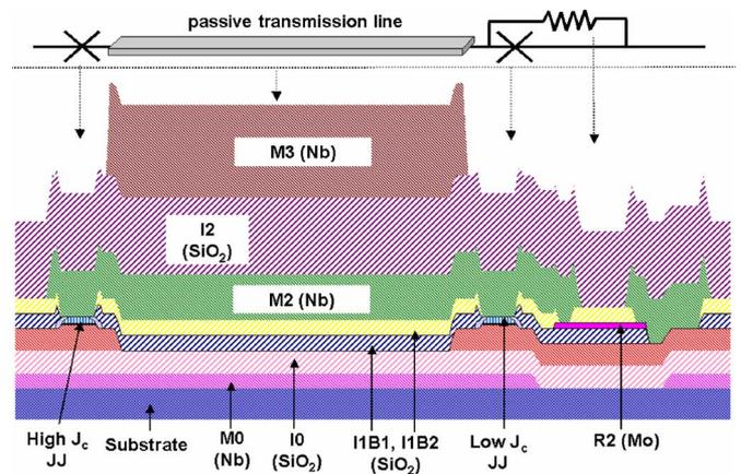
Fig. 4. The final cross-section of the driver receiver pair. A passive transmission line connecting the two outer JJs.
