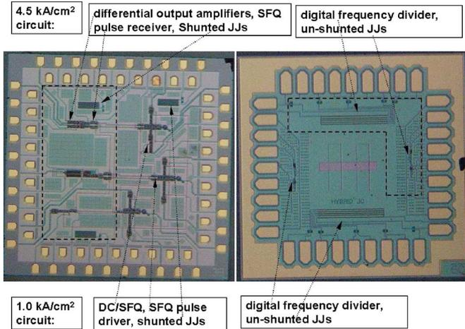
Fig. 5. Dual- $J_c$  (1 and 4.5  $\text{kA}/\text{cm}^2$ ) chips, the area enclosed by the dashed-lines is for  $J_c = 4.5 \text{ kA}/\text{cm}^2$ .
