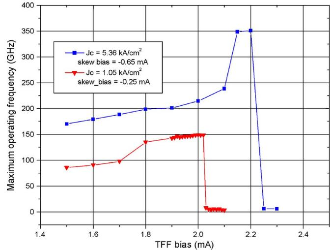
Fig. 7. The maximum operating frequency of the digital frequency divider vs. the TFF bias (mA) fabricated by a multi- $J_c$  process on the same chip.
