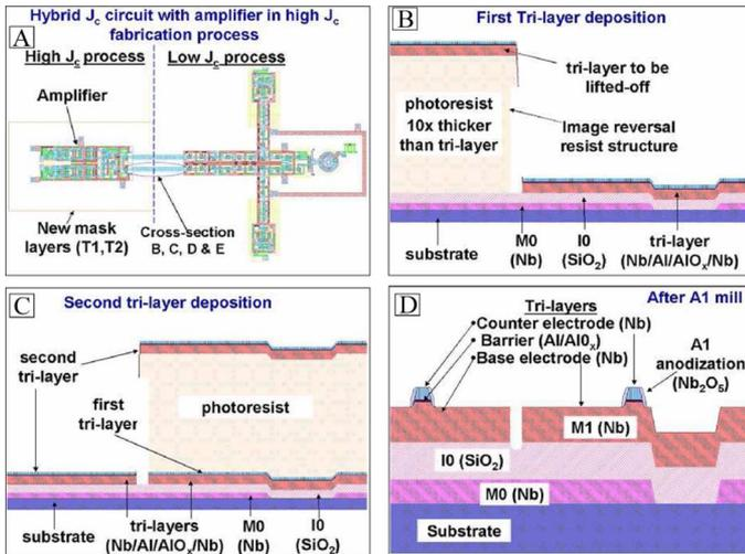
Fig. 3. Multi- $J_c$  fabrication process for a typical digital circuit. (a) Circuit layout for the low and high- $J_c$  parts and the driver/receiver pair between the two parts. (b), (c) and (d) the cross-section of the driver/receiver pair after the deposition of the first trilayer, deposition of the second trilayer, and the junction definition steps respectively.
