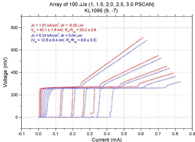
Fig. 6. Arrays of 100 unshunted JJs of sizes ranging from 1.0 to 3.0 PSCAN with dotted and solid lines for 1.0  $\text{kA}/\text{cm}^2$  and 4.5  $\text{kA}/\text{cm}^2$  respectively.
