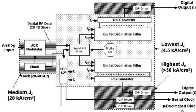
Fig. 1. Tri- $J_c$  digital-RF receiver architecture concept: complex part with more than  $10^4$  JJs (Digital I/Q decimation filter, mixer, LO—local oscillator, PS—parallel to serial converter) to be implemented in the lowest- $J_c$ ; the clock source and ADC modulator to be implemented in medium- $J_c$ , and all the high voltage drivers to be implemented in the highest possible  $J_c$ .
