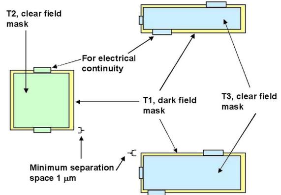
Fig. 2. Layout of the three additional photomasks required for processing the circuit architecture described in Fig. 1. Mask “T1”—dark field, “T2”, “T3”—clear field for the lowest, medium and highest- $J_c$  processes, respectively.
