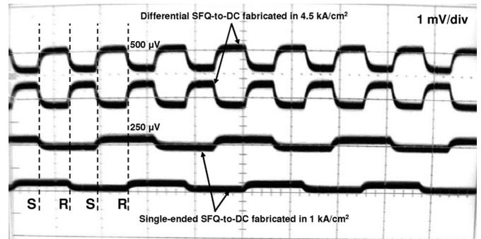
Fig. 8. Low speed test results for the differential SFQ-to-DC amplifier, showing the doubling of signal speed and amplitude as it traverses from the 1  $\text{kA}/\text{cm}^2$  to the 4.5  $\text{kA}/\text{cm}^2$  part of the circuit.
