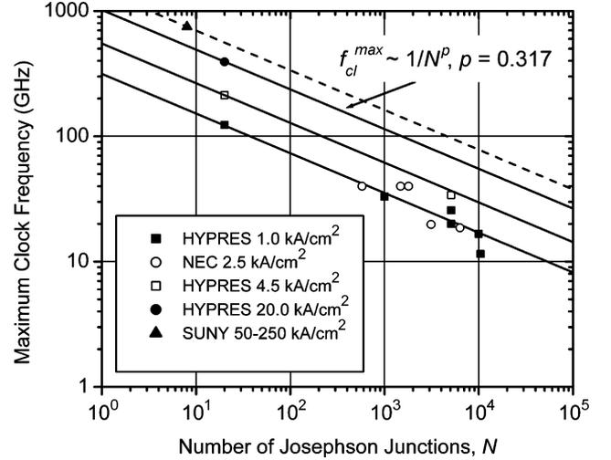
Fig. 7. Dependences of the maximum clock speed of RSFQ digital circuits on the number of Josephson junctions for the existing and projected Nb fabrication processes. The experimental data are from this work and [7], [8], [11]–[13]. The data for NEC process are from [3], [20]–[23]. Solid lines show the best fit to the data on 1 and 4.5  $\text{kA}/\text{cm}^2$  processes, and projections for the 20 and a hypothetical 250  $\text{kA}/\text{cm}^2$  (dash line) processes.
