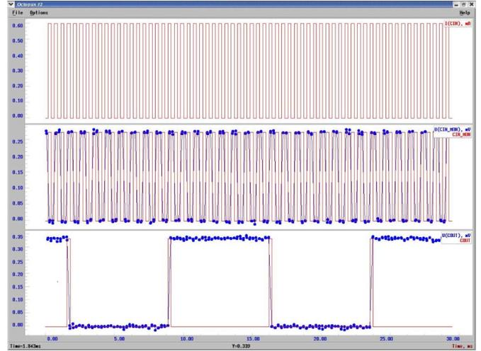
Fig. 5. Digital low-speed testing of the  $20 \text{ kA/cm}^2$  4-bit digital counter. The panels show from top to bottom the applied pattern, the input SFQ/DC monitor, and the counter output, respectively. Bias margins are  $\pm 27\%$ .
