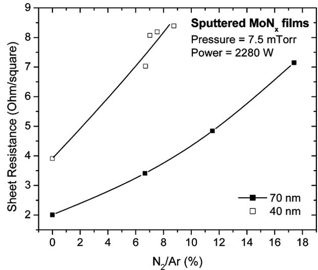
Fig. 1. Average sheet resistance of MoN<sub>x</sub> films at room temperature as a function of N<sub>2</sub>/Ar ratio in the sputtering mixture. The pallet scan speed was adjusted to provide the MoN<sub>x</sub> film thicknesses of 70 nm and 40 nm. Data points are connected to guide the eye.
