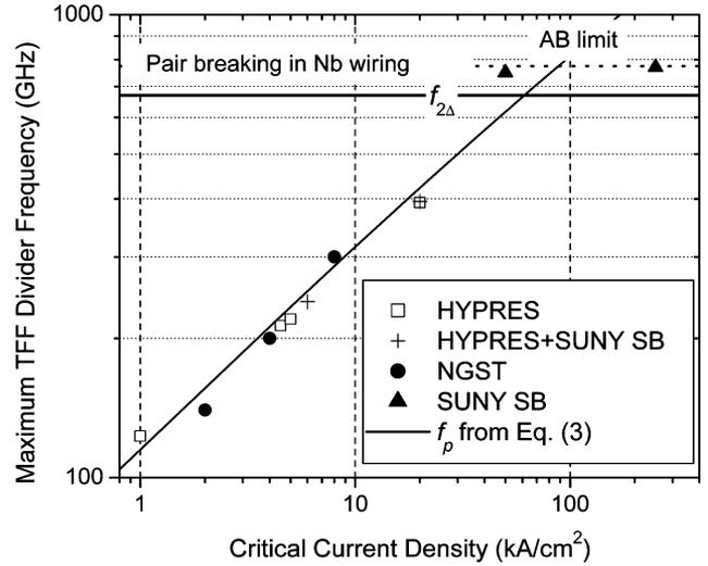
Fig. 6. Maximum frequency of operation of TFF-based frequency dividers fabricated in various Nb-based processes. HYPRES data are from the present work and [18]; HYPRES+SUNY SB data are from [18]; NGST data are from [14]; SUNY SB data are from [7], [8]. Above the gap frequency of Nb ( $\sim 670$  GHz) strong attenuation of SFQ pulses in Nb wiring and JJ electrodes should set in. The JJ plasma frequency  $f_p$  (3) is shown as a solid curve, AB limit as a dotted line.
