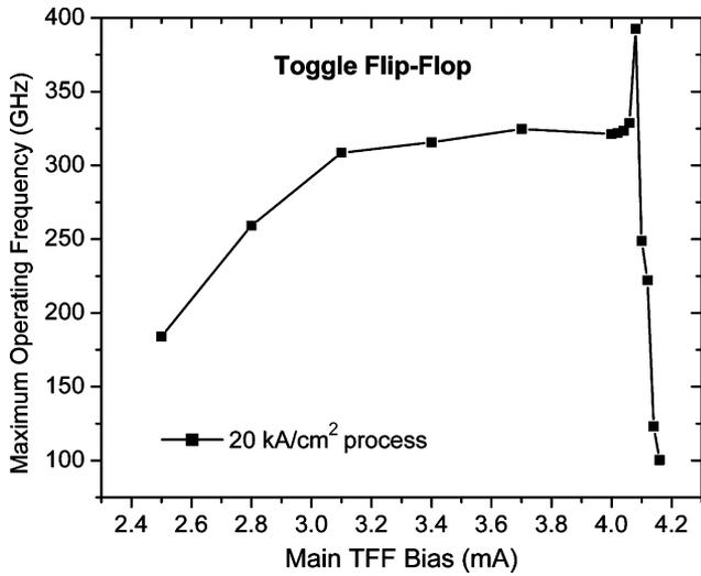
Fig. 4. Maximum operating frequency  $f_{max}$ , of the Toggle Flip-Flop (static frequency divider) as a function of the circuit's main bias. The absolute maximum corresponds to  $f_{max} = 393$  GHz, whereas the widest margins of operation correspond to  $\sim 325$  GHz input frequency.
