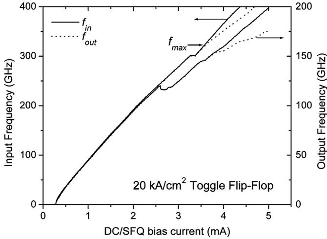
Fig. 3. Input frequency of the TFF (solid curves, left scale as indicated by arrow) and output frequency (dotted curves, right scale as indicated by arrow) as a function of the input bias current. The upper and the lower pair of curves correspond to the main TFF biases of 4.06 mA and 3.10 mA, respectively. The maximum operating frequency at a given bias,  $f_{max}$  corresponds to the point where  $2 \cdot f_{out}$  starts to deviate from  $f_{in}$  (divide by two operation fails).
