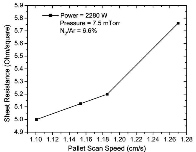
Fig. 2. Average sheet resistance of MoN<sub>x</sub> films at room temperature as a function of the pallet scan speed during reactive sputtering in N<sub>2</sub> + Ar mixture. The thickness of the films changes from 55 nm to 46 nm and scales inversely with the pallet speed. Data points are connected to guide the eye.
