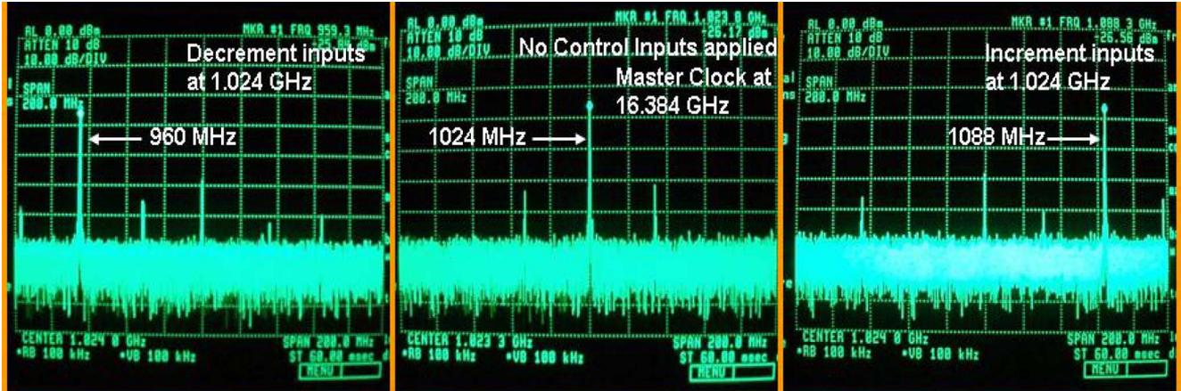
Fig. 11. Frequency spectrum of the phase rotator output at 16.384 GHz master clock. The center spectrum represents absence of control inputs, whereas the right and left spectra are in the presence of increment and decrement inputs respectively.
