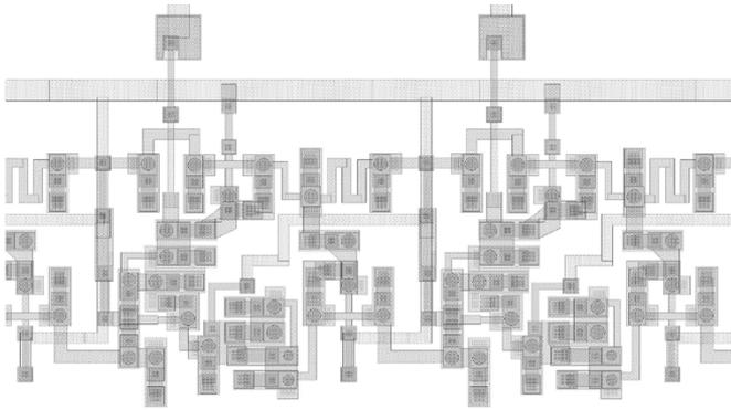
Fig. 8. Layout fragment of 2 bits of the programmable frequency divider.
