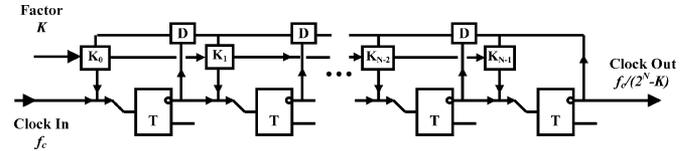
Fig. 6. Block diagram of the programmable frequency divider.
