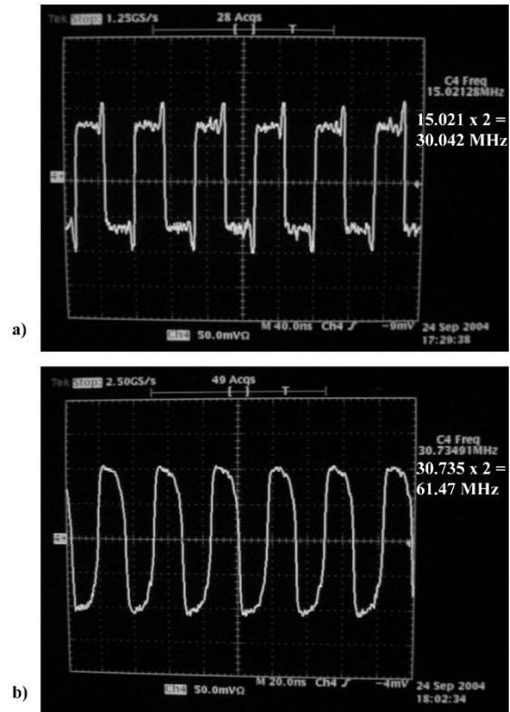
Fig. 10. HF test of the programmable frequency divider at 30.72 GHz. With decimation (a) by 1024 ( $K = 0$ ) and (b) by 500 ( $K = 524$ ).
