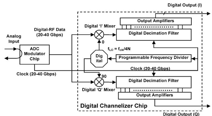
Fig. 1. Block diagram of a channelizing digital receiver.
