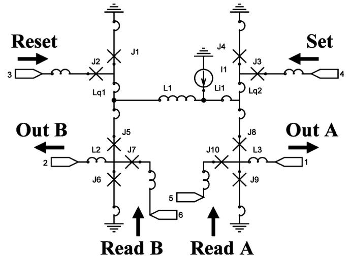
Fig. 14. Schematics of the dual-port NDRO cell.
