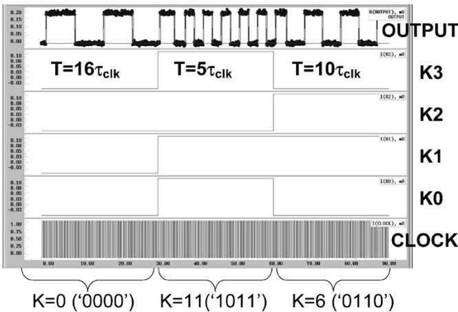
Fig. 9. Functionality test of the 4-bit programmable frequency divider.
