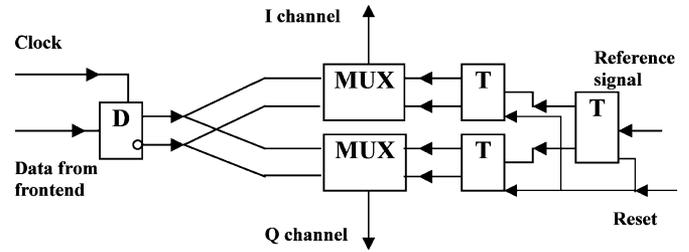
Fig. 13. Block-diagram of a novel digital I/Q square-wave mixer.
