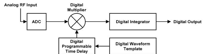
Fig. 2. Block diagram of a generic correlation-based digital receiver.
