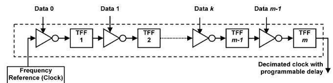
Fig. 3. Block diagram of programmable phase generator.
