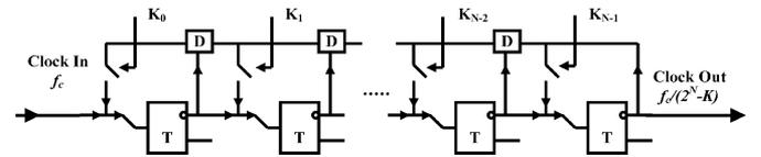
Fig. 7. Block diagram of a simplified version of the PFD.
