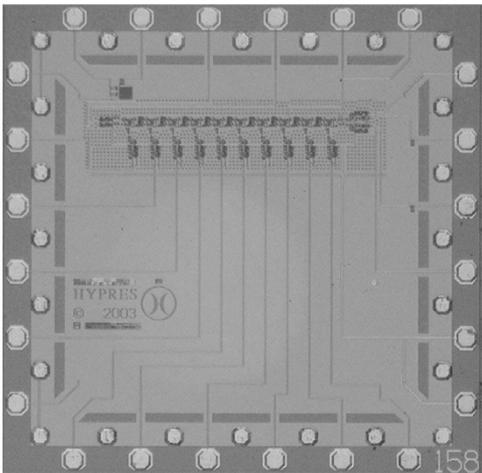
Fig. 5. Photograph of a 5-mm chip fabricated using HYPRES' 1 kA/cm<sup>2</sup> process with a 10-bit programmable phase generator.
