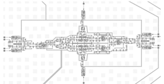
Fig. 15. Layout of digital I/Q mixer.
