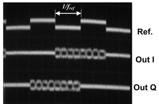
Fig. 18. High-speed test of the mixer. Clock—40.0 GHz, Data—10.000 01 GHz, Reference—10 kHz.
