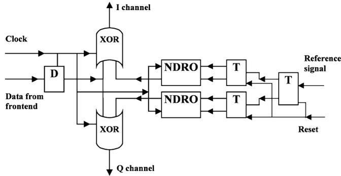
Fig. 12. Block-diagram of the digital I/Q square-wave mixer.
