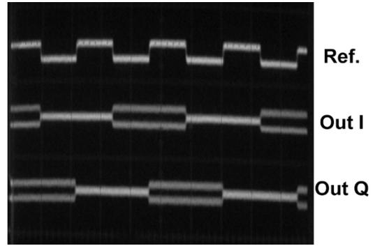
Fig. 17. High-speed test of the mixer at maximum negative slew rate signal case. Clock—42 GHz, no Data, Reference—20 kHz.
