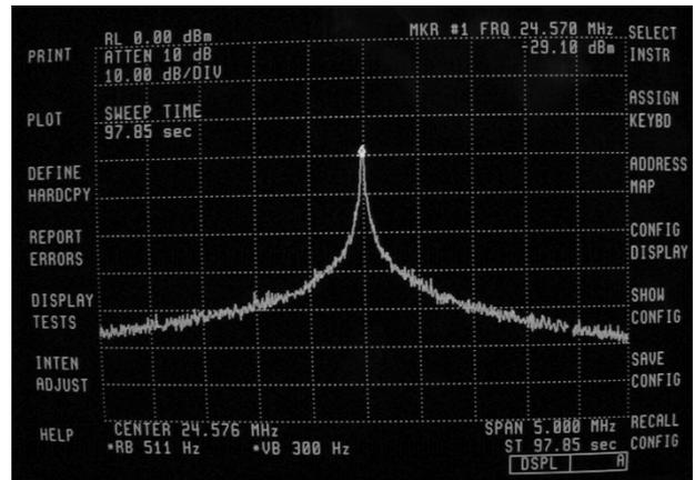
Fig. 11. HF test of the 10-bit PFD with spectrum analyzer.
