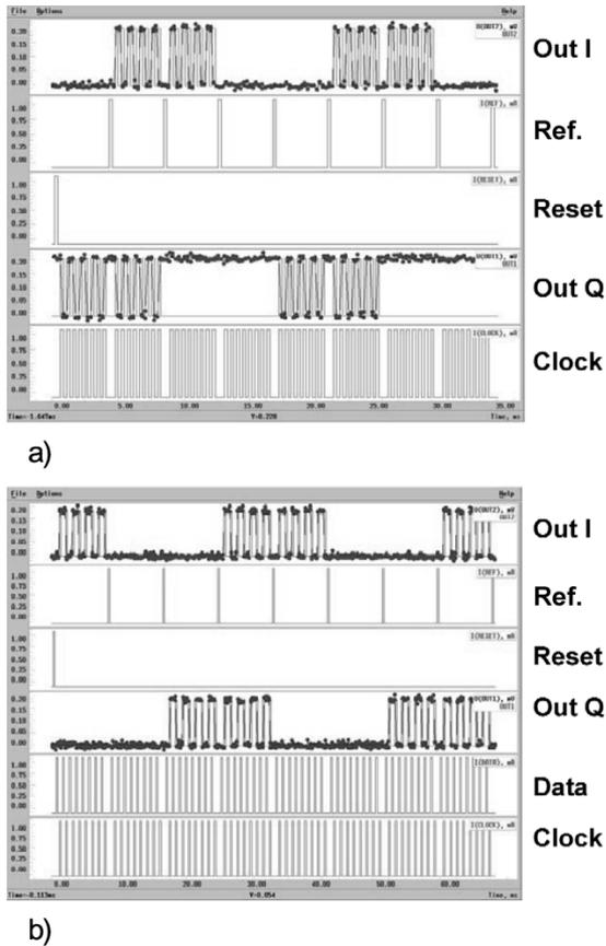
Fig. 16. Low-speed functionality test of the mixer, with maximum negative slew rate signal (a) and maximum positive slew rate signal (b).
