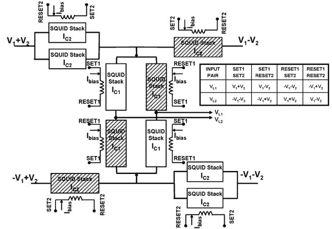
Fig. 6. Differential digital amplifier featuring dynamic equalization. RSDCA and other control circuitry are not shown. Table shows the voltages at respective outputs for different combinations of SET and RESET signals.
