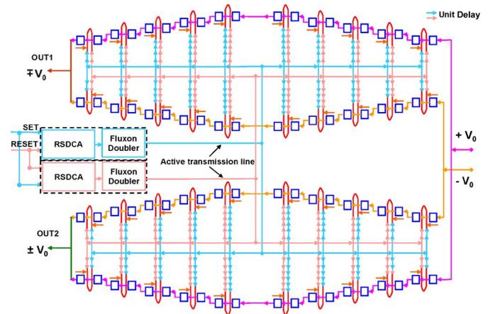
Fig. 11. Schematic of the H-Tree amplifier with triangular heads. Equalized propagation time of the control signal to each SQUID.
