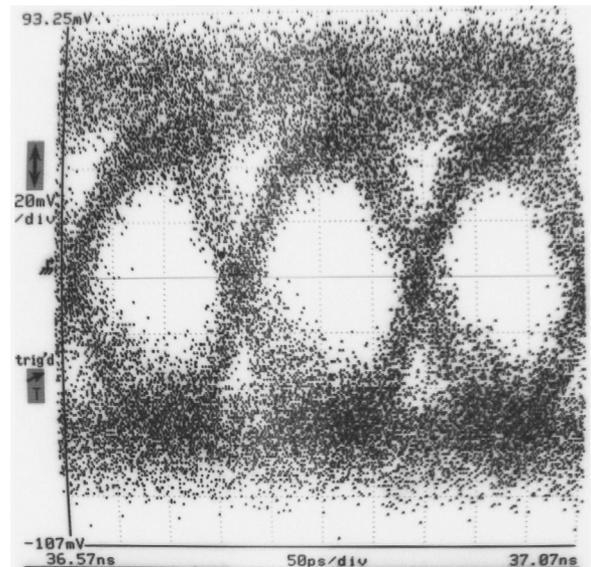
Fig. 16. Eye-diagram measurement for the half H-Tree amplifier. Only one of the differential outputs is followed by the SHF LNA.
