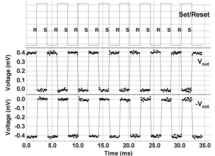
Fig. 18. Low speed test result for differential SFQ-to-DC digital amplifier. The amplifier exhibits  $800 \mu\text{V}$  differential output.
