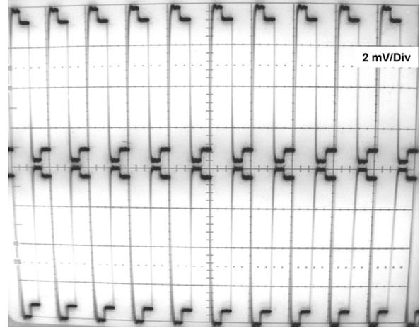
Fig. 8. Low speed test result for the amplifier with pre-emphasis. The amplifier exhibits 16 mV differential output.
