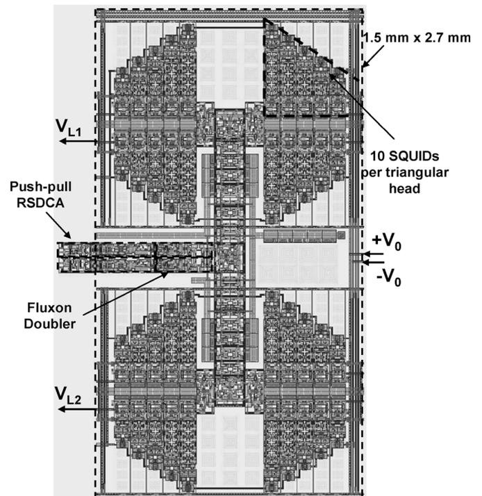
Fig. 12. Layout of half H-Tree amplifier.
