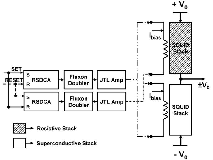
Fig. 3. Functional schematic of the bipolar single-ended digital amplifier. The structure consists of two SQUID stacks driven by control signals SET and RESET such that one stack remains in resistive state while the other stack remains in superconductive state. The superconductive stack provides a loss less path from the applied voltage to the output.
