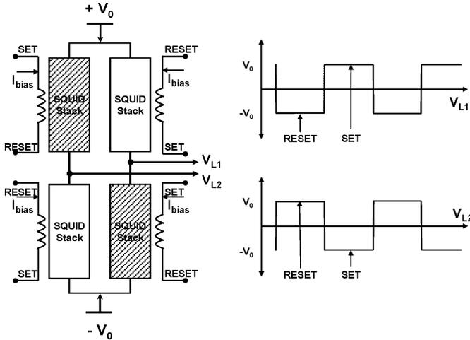
Fig. 4. Functional schematic (left) of bipolar differential digital amplifier. SET, RESET signals chosen to place a diagonal pair of stacks in resistive state while the other diagonal pair in superconductive state. Expected waveforms for the SET, RESET inputs shown on the right.
