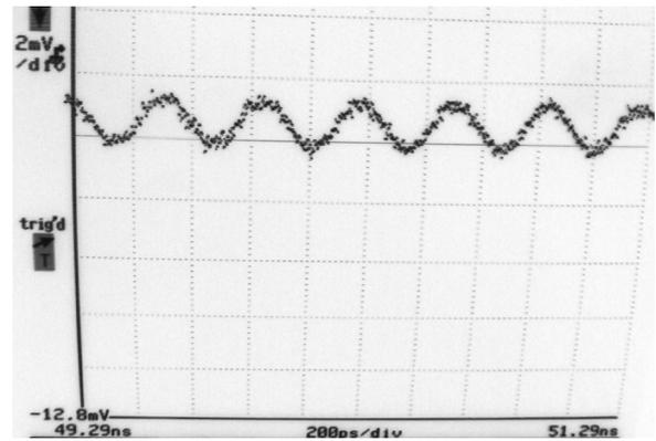
Fig. 9. High speed test result for the amplifier with pre-emphasis. Only one output is shown in the figure. Input data applied without consecutive transition (“1100” pattern).
