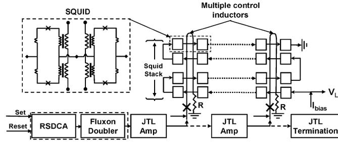
Fig. 1. Functional schematic of improved unipolar single-ended digital amplifier based on SQUIDs modulated by multiple control inductors coupling flux into the SQUID loops.
