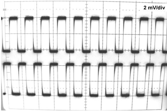
Fig. 13. Low speed test result for the Half H-Tree amplifier. The amplifier exhibits 8 mV differential output.
