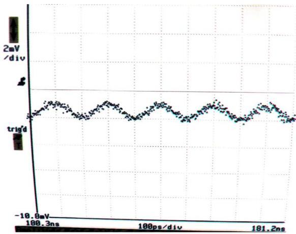
Fig. 14. High speed test result for the half H-Tree amplifier. Only one of the two outputs shown in the figure.
