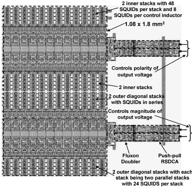
Fig. 7. Layout of differential digital amplifier featuring dynamic equalization.
