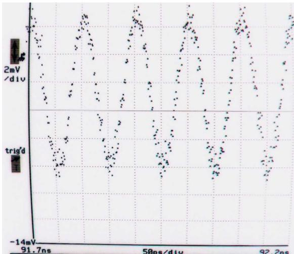
Fig. 19. High speed test result for the differential SFQ-to-DC amplifier. A single output is further amplified by a MITEQ amplifier with a 40 dB gain at room temperature.
