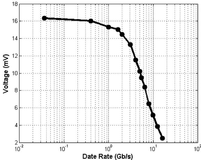
Fig. 10. High speed response of the differential amplifier featuring dynamic equalization.
