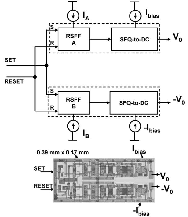
Fig. 17. Differential SFQ-to-DC digital amplifier. Inset below shows the layout of the amplifier.
