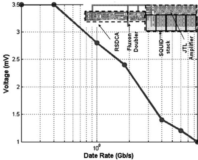
Fig. 2. High speed response for the improved unipolar single-ended digital amplifier. Inset shows the layout of the amplifier.
