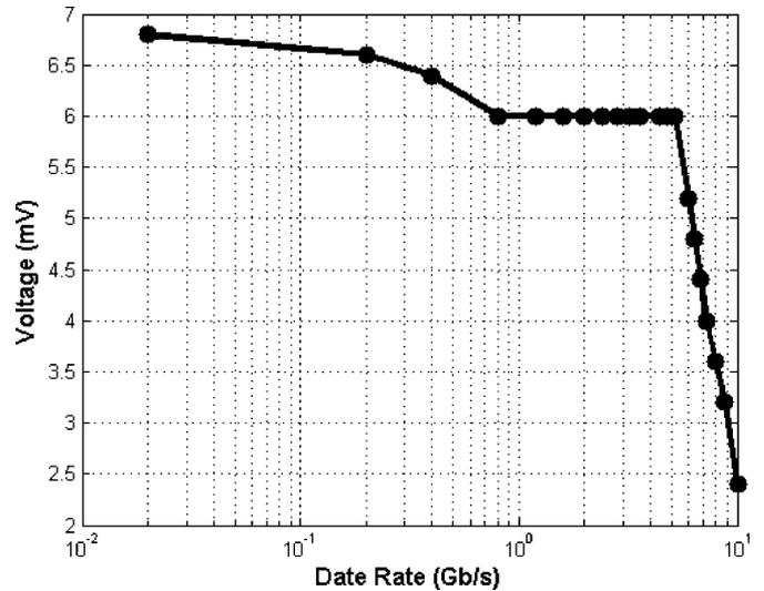
Fig. 15. High speed response of the half H-Tree differential amplifier.
