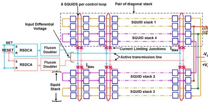
Fig. 5. Schematic of the bipolar differential digital amplifier designed to work in a push-pull configuration with equal rise and fall times.
