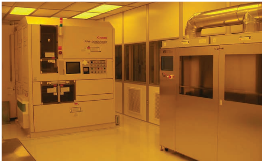
3. The new six-layer superconducting circuit process is made possible with a 5X reduction stepper system from Canon ( www.canon.com ) which can fabricate device features as fine as 250 nm.
