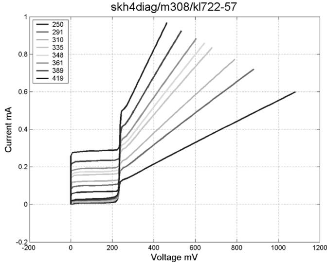
Fig. 3. The typical  $IV$  curves of 100-junction arrays of circular junctions. The on-chip diameter of the junctions is from  $3.5$  to  $1.5 \mu\text{m}$  from top to bottom.
