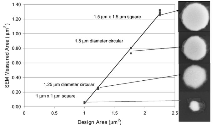
Fig. 2. SEM-measured area vs. design area for square and circular junctions of designed size of 1.5 μm and less, features patterned on 2000 Å of Nb.
