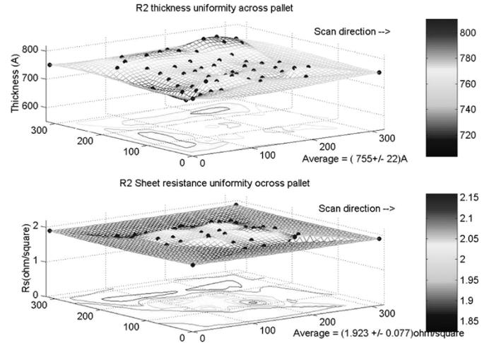
Fig. 5. The sheet resistance and resistor layer thickness uniformity across  $300 \times 300 \text{ mm}$  pallet. The sheet resistance was measured using a 4-point resistance probe while thickness was measured using a stylus profilometer.
