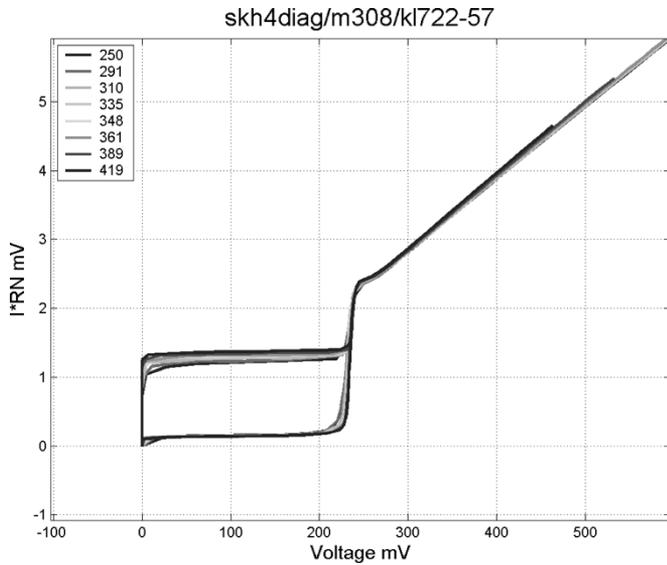
Fig. 4. Normalized  $IV$  curves for the same arrays as in Fig. 3. The critical current spread across the chip is about  $2.4\%$  as compared to the spread in individual arrays of less than  $1.2\%$ .
