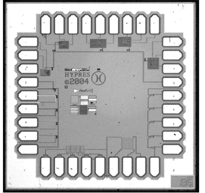
Fig. 1. The typical process monitoring chip for inductances, junction specific capacitance, sheet resistance and resistors over-etch.
