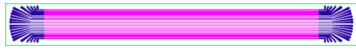
Fig. 2. Mask for ion-beam milling 100 mm-long by 12 mm-wide YBCO tape sample. Lines are darker at each end showing the region of silver coating.
