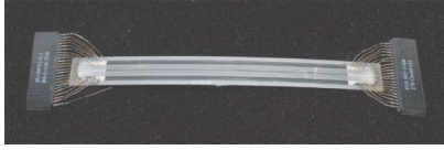
Fig. 3. 100 mm-long by 12 mm-wide tape with 22 lines of various widths and separations. 24-pin connectors are soldered directly to the silver-coated pads.
