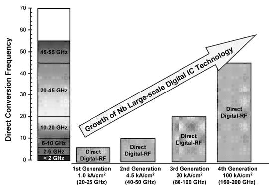
**Fig. 3** Expected progress of directly digitizing Digital-RF systems with better fabrication process.
