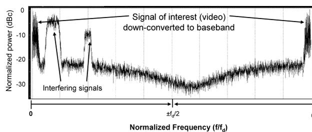
**Fig. 20** The X-band ADR system operation. The measured spectrum of the received satellite signal-of-interest with input 7676 MHz signal modulated at 1.544 Mbps with a packetized video file. Our wideband XADR receiver also captured other signals in the same transmitted band, at 7679 MHz and 7684 MHz. The clock frequency is  $\sim 10.235$  GHz.
