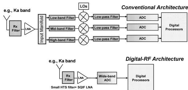
**Fig. 1** Comparison of conventional and Digital-RF receiver architectures.
