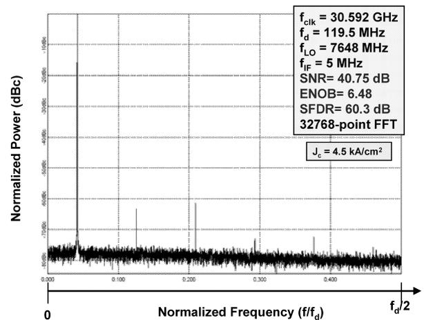
Fig. 5 Spectrum of the digitized output from an X-band ADC chip clocked above 30 GHz. The chip consisting of a band-pass ADC modulator, digital mixer and digital filter. The applied analog input signal is 7.653 GHz.
