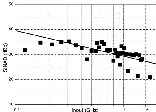
**Fig. 17** The HF/L-band ADR system test. SINAD vs. input signal frequency. Line with the slope of 3 dB/octave is also shown.
