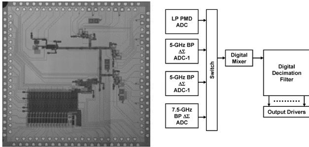
**Fig. 11** Multi-band Digital-RF receiver test chip. Microphotograph of a  $10 \times 10 \text{ mm}^2$  (left) and block diagram (right) of a circuit with four different ADC modulators connected to a single mixer and filter.
