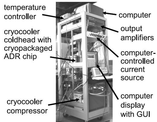
**Fig. 13** Fully equipped 19-inch rack with all components of digital receiver system based on Sumitomo 4 K cryocooler.
