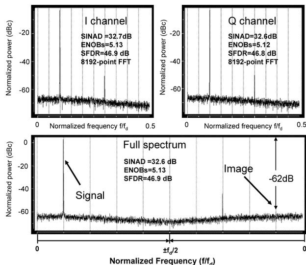
**Fig. 19** The X-band ADR system test. The spectra of the I-channel output (top left), the Q-channel output (top right) along with the full 8192-point spectrum (I+jQ, bottom) acquired at 10.24 GHz. The input tone frequency is 7676 MHz. The LO is 2560 MHz to mix with signal alias at 2564 MHz (IF is 4 MHz). The output bandwidth ( $f_d = f_{clk}/256$ ) is 40 MHz.
