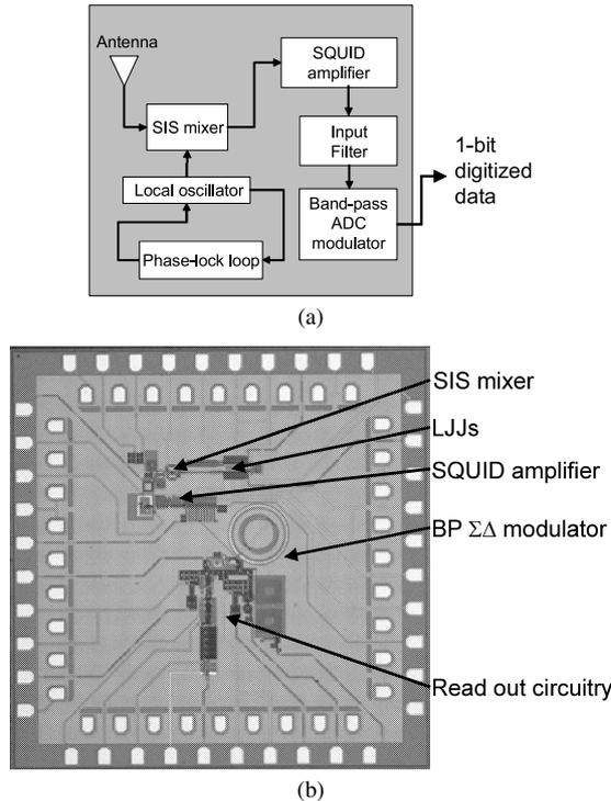
**Fig. 6** A mm/submm signal digitizer designed for 350 GHz input signal. (a) block diagram. (b) a microphotograph of the mm/submm digitizer test chip ( $5 \times 5 \text{ mm}^2$ ).
