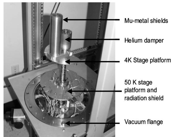
**Fig. 14** View of open cryostat with ADR cryopackage mounted on cryocooler coldhead.
