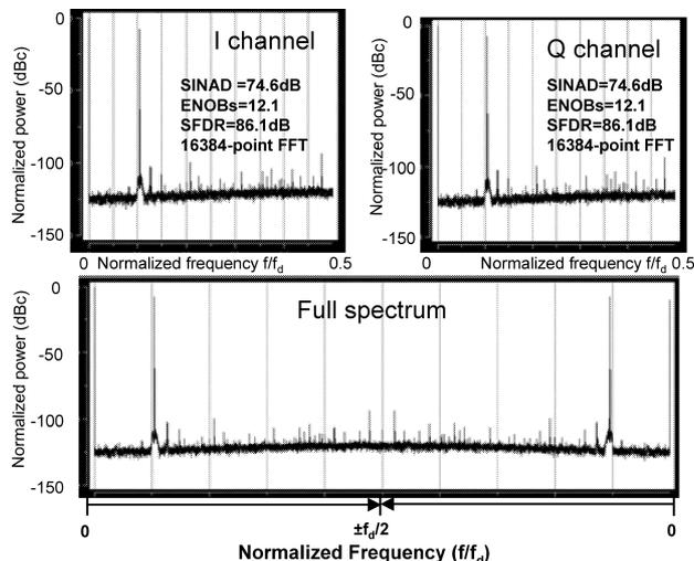
**Fig. 15** The HF/L-band ADR system test. Measured spectrum of the digital I and Q data and complex I+jQ FFT for a single 10 MHz tone input sampled at 24.32 GHz clock, digitally filtered, and acquired to FPGA at 95 MS/s.
