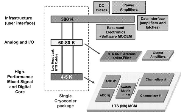
**Fig. 12** Hybrid Temperature Hybrid Technology ( $ht^2$ ) system integration approach.
