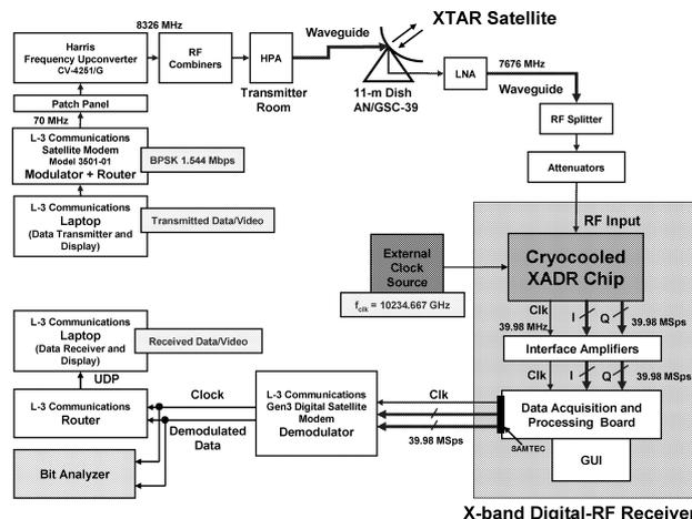
**Fig. 18** Block diagram of X-band ADR system demonstration with live XTAR satellite.
