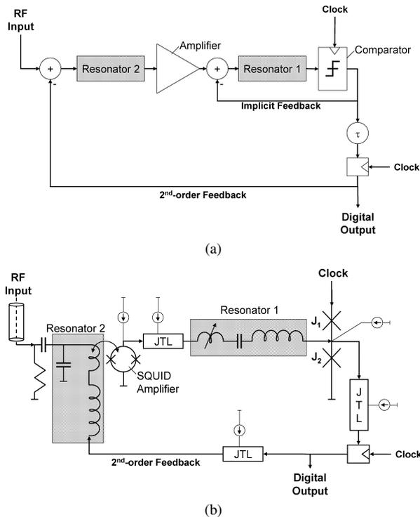
Fig. 4 Second-order bandpass  $\Delta\Sigma$  ADC modulator. (a) Block diagram. (b) Schematics.
