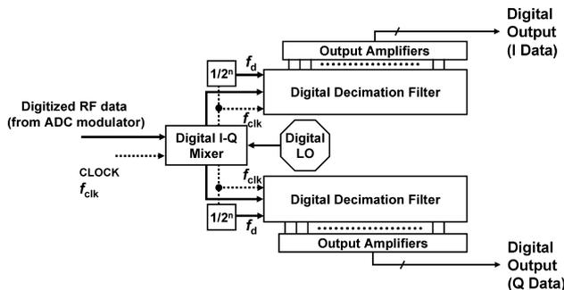
**Fig. 7** Block diagram of a single channel of digital channelizer comprising a digital in-phase (I) and quadrature (Q) digital mixer and two digital decimation filters.
