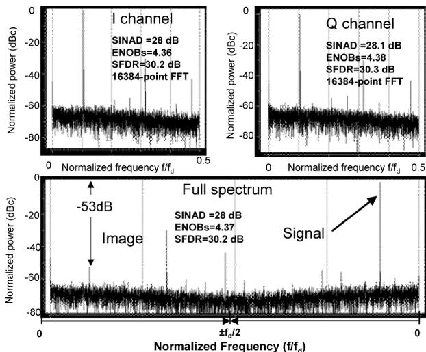
**Fig. 16** The HF/L-band ADR system test. The spectra of the I-channel output (top left), the Q-channel output (top right) along with the full 32768-point spectrum (I+Q, bottom) acquired at 24.32 GHz. The input tone frequency is 1.5 GHz and the LO is 1.49 GHz. The output bandwidth ( $f_d = f_{clk}/256$ ) is 95 MHz.
