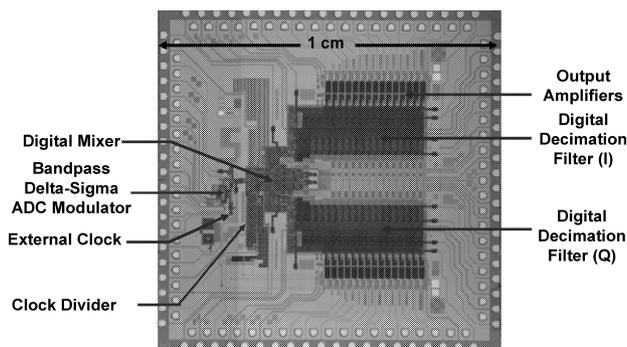
**Fig. 10** Microphotograph of a single-channel superconductor X-band Digital-RF receiver chip (XADR). This 10 × 10 mm<sup>2</sup> chip is fabricated using HYPRES 4.5 kA/cm<sup>2</sup> process and comprises about 11,000 Josephson junctions.
