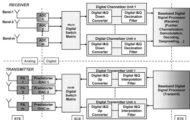
**Fig. 2** Block diagram of a programmable multi-band, multi-channel Digital-RF Transceiver. It employs a combination of cryogenic superconductor electronics (SCE) and room-temperature electronics (RTE) elements located on different temperature stages of a cryocooler.
