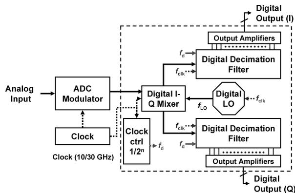
**Fig. 9** Block diagram of digital-RF receiver chip (ADR chip) integrating ADC modulator and digital channelizer on a single chip.
