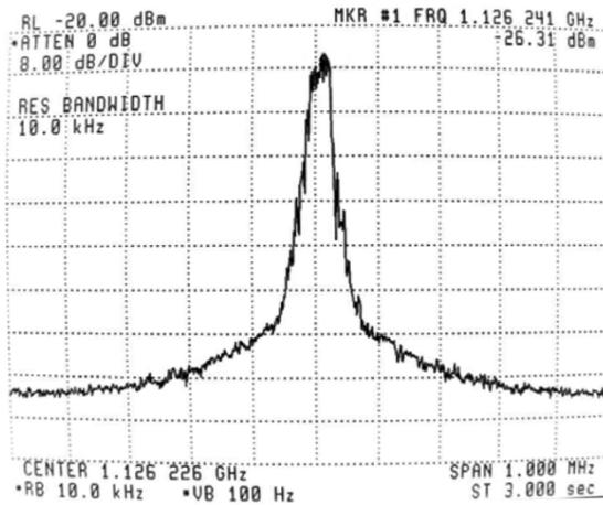
Fig. 6. The spectrum of free running annular LJJ set up at  $f = 36$  GHz.
