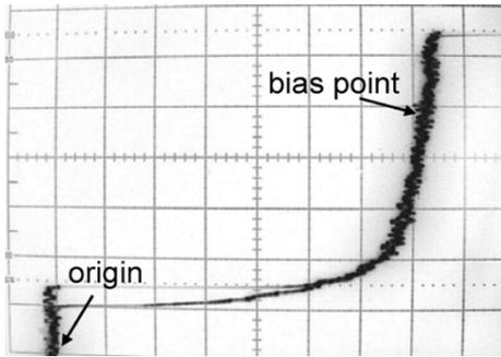
Fig. 5. The I-V curve of annular Josephson junction with 10.4 mA control current. The horizontal and vertical scales are 10 mV/div and 1 mA/div.
