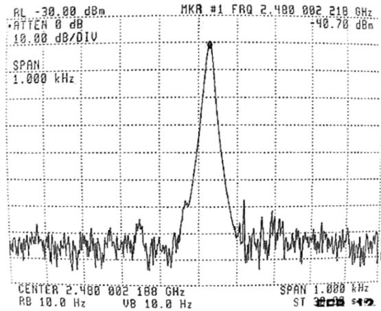
Fig. 7. The spectrum of annular LJJ set up at  $f = 39.7$  GHz. The junction was phase-locked to 16th harmonic of room temperature synthesizer set up at 2.48 GHz and fed to the junction through bias lead.
