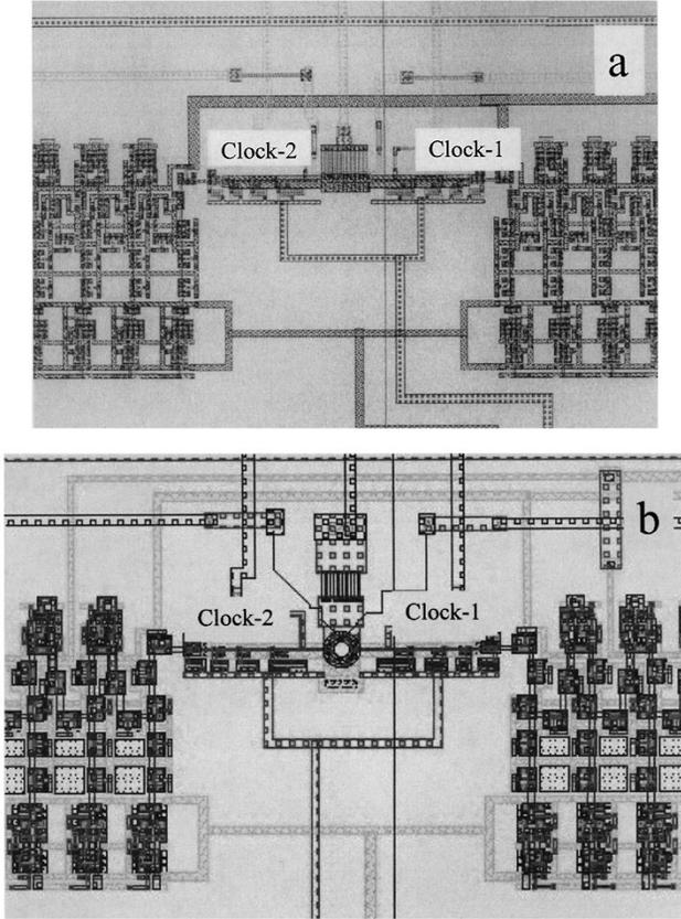
Fig. 2. The layouts of (a) linear and (b) annular LJJ oscillator coupled through two interface JTL's to two chains of binary frequency dividers (only first two dividers are shown for the clarity) on both ends.
