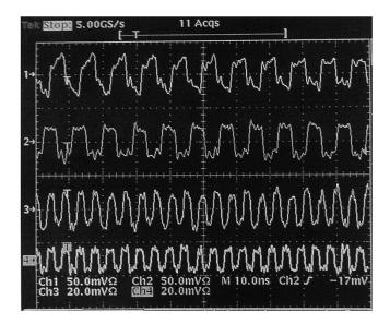
Fig. 4. The waveforms of four outputs from linear LJJ. The frequencies are the following: output 1—111.11 MHz, output 2—113.63 MHz, output 3—221.42 MHz, output 4—227.27 MHz. LJJ is biased on the first ZFS.
