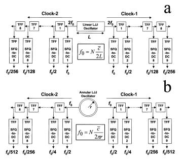
Fig. 3. Block diagram of the two phase clock generator using (a) linear and (b) annular LJJ.
