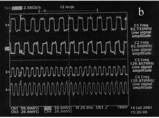
Fig. 5. The waveforms of four outputs from annular LJJ. LJJ is biased on the first ZFS with (a) 2.31 mA current and (b) 4.2 mA current, corresponding to the bottom and the top of the ZFS respectively.
