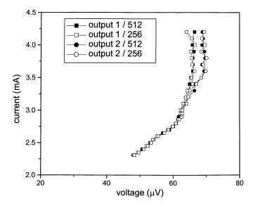
Fig. 6. The first zero-field step of the current-voltage characteristics of the annular LJJ, reconstructed from the frequency measurements.
