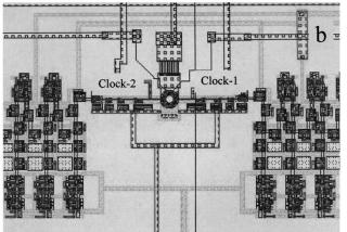
Fig. 2. The layouts of (a) linear and (b) annular LJJ oscillator coupled through two interface JTL's to two chains of binary frequency dividers (only first two dividers are shown for the clarity) on both ends.
